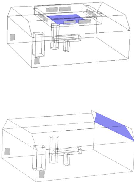
**Figure 1.** Operation room with Laminar Air-flow ventilation (top) and mixed ventilation (bottom). Air comes in through the blue areas and leave the room in the grey areas. Operation table, surgeon (cylinder) and equipment next to the operation table are also indicated.
