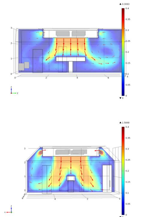
**Figure 3.** Two cross-sections of the air-flow in the laminar air-flow design. Air (red arrows) move down from the overhead inlet and moves out through the (grey) outlets. Notice that the unsymmetrical position of these makes a vortice to the right. The color coding is in m/s.
