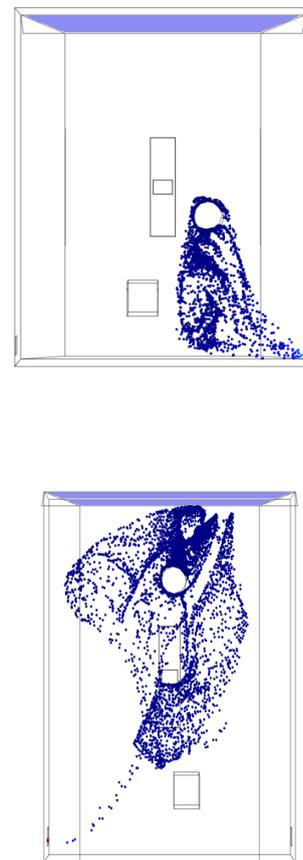
**Figure 7.** Particle positions after one minute after release for the mixed ventilation case. The top figure shows the wanted outcome when the surgeon is at the side of the operation table and the bottom figure the dramatic disturbance of the flow when a person is standing between the table and the inlet.
