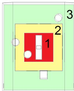
**Figure 4.** Suggested division of the operation room into three zones. The red zone is the most critical one corresponding to the size of the air inlet feature, while zone 2 and especially 3 has less influence on the air-flow around the patient. Zone 2 corresponds to the air outlets in the roof.
