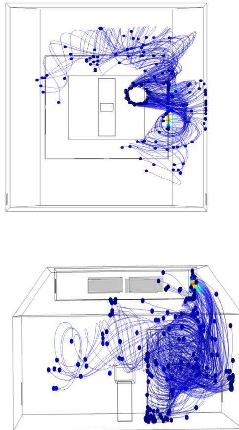
**Figure 5.** Particle trajectories in the laminar air-flow situation. Top shows particle positions (blue dots) after two minutes and their trajectories. Bottom the same from the side instead of from above.
