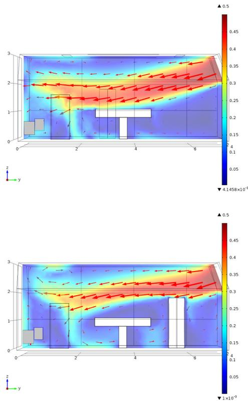
**Figure 6.** Two cross-sections of the air-flow in the laminar air-flow design. Air (red arrows) move down from the inlet to the right and moves out through the (grey) outlets. The color coding is in m/s. The bottom figure shows the air-flow when a person is standing next to the operating table on the right hand side.
