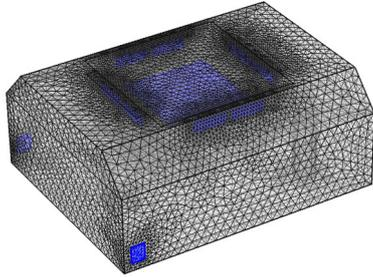
**Figure 2.** Calculational mesh for the operation room with Laminar air flow ventilation; blue areas indicate air inlets and outlets.
