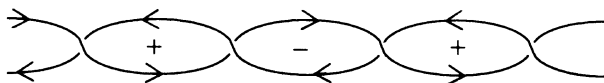
Fig. 3 A TP cable is a series of magnetic dipoles that will cancel each other pair wise.
