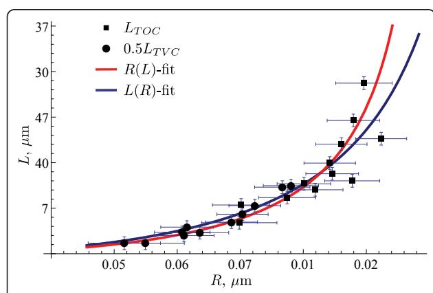
**Figure 4 Comparison of experimental and model results (unified description).** The measurement points (shown as markers) for both TVC and TOC plotted after dividing the TVC length by two. Parameters for the model predictions were chosen to minimize functionals (11) (red line) and (10) (blue line).
