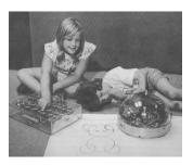
The robot has a set of pens or crayons of different colours, which it can switch between. It can lift the pen (for not drawing) or lower it (for drawing). It can move forward and backward, and turn right and left. The robot can also be programmed to execute command sequences; e.g., it is possible to define that a "square" is to first move forward, turn left 90 degrees, and then redo the same thing three more times.
