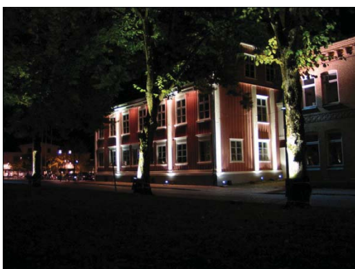
Figure 6. Façade and tree trunks with uplight.
