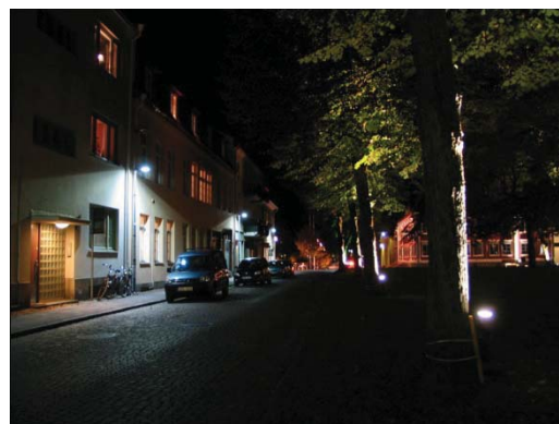
Figure 2. Street light at 4.5 metres height.
