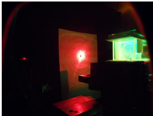
Fig. 4. An image of the Fraunhofer diffraction pattern used to determine of the size of the droplet.
