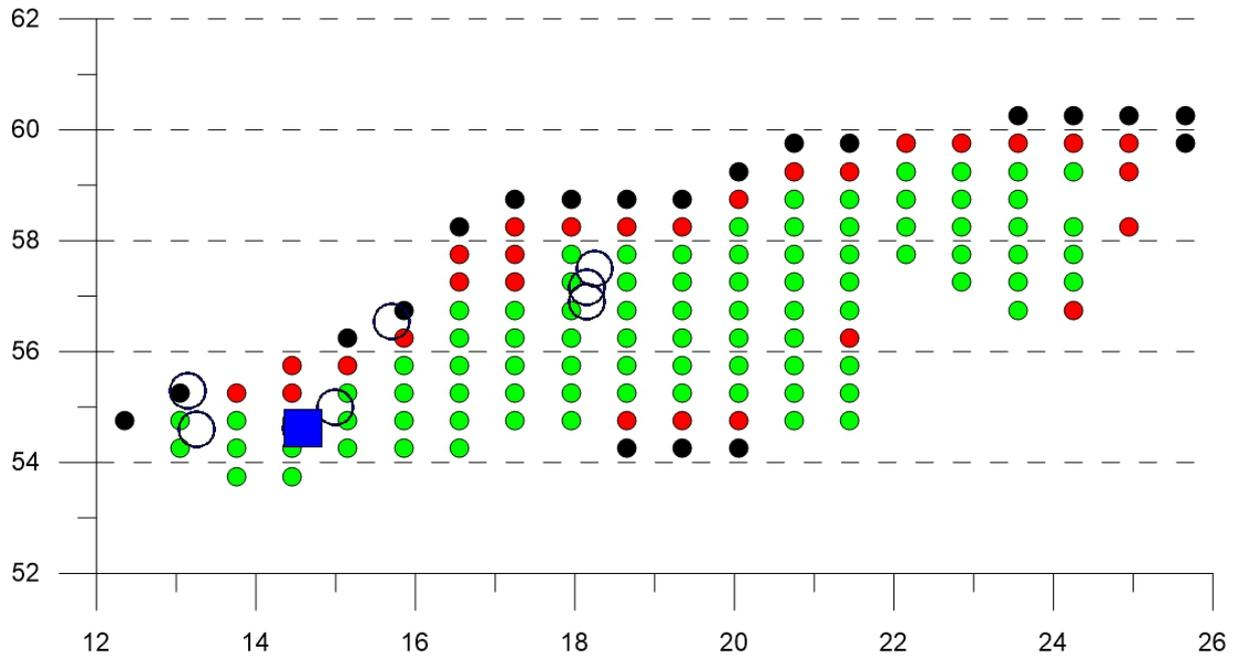
*Frequency of a trajectory passing through the boxes of  $0.7^\circ \times 0.5^\circ$  size – green: often, red: sometimes, and black: rarely. Point of release. Blue box, points of finding: open blue circles. Horizontal axis: degrees longitude vertical axis: degrees latitude.*
