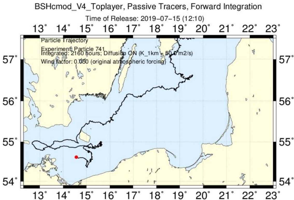
*Two simulated trajectories, emanating from the red dot, extending across 90 days. A random displacement, accounting for the lack of sufficient small-scale turbulent movement, is added, and responsible for the wiggly development. Note that this trajectory is not passing any of the findings spots. – 2<sup>nd</sup> diagram for alternative trajectory needed*
