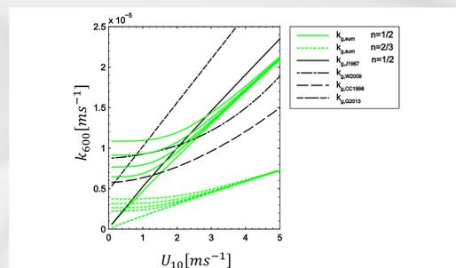
Figure 3. Transfer velocity constant  $k_{g,600}$  according to equation (23) in green for  $Q_0 = 0, 50, 100, 200$  and  $400 \text{ Wm}^{-2}$  and  $n = 1/2$  (clean) and dotted line  $n = 2/3$  (saturated surfactant). The parameterizations in equations (2-5) are given for reference. The transfer velocity estimated with equation (4) is transformed into  $Sc = 600$  using  $k_{g,Sc_1} = k_{g,Sc_2} (Sc_1/Sc_2)^{-n}$  and  $n = 1/2$ .
