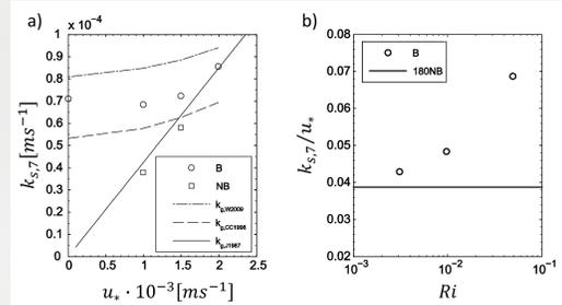
Figure 2. a) The scalar transfer velocity  $k_{s,7} = k_{s,7}/\Delta S_{s,c}$ . Circles denote cases with buoyancy and squares denote no-buoyancy cases. The dashed and dash-dotted lines denote the wind parameterizations with  $n = 1/2$  according to equations (3) and (4) respectively. The solid line denotes a linear increase of the transfer velocity as a function of the friction velocity (2). b) Transfer velocity constant  $k_{s,7}/u_*$  as a function of  $Ri$ .
