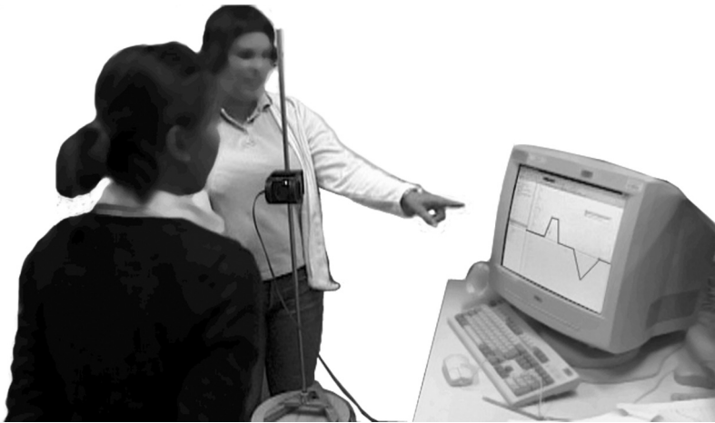
Figure 1. Probeware. Two students interacting with the motion sensor (left) and the interface (right).
