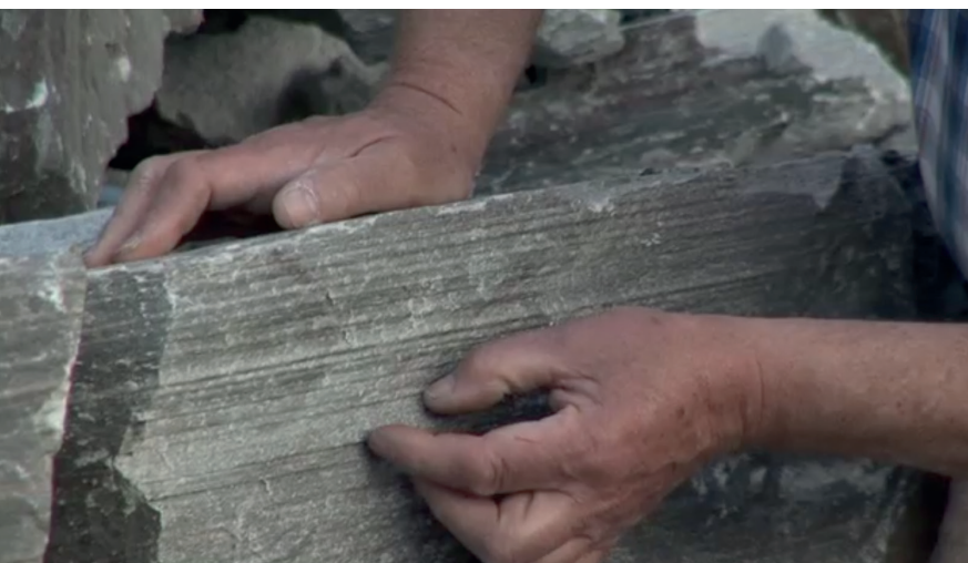
Fig 15-16. Sigvard Nyström in action in Glava Quarry, cleaving the shale slab into roofing shingles. His judgments of sound direct his actions. Pictures from the film.
