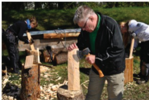
Figure 3. Parishioners, local craftsmen and conservation officers participated in the co-production of wooden shingles. Photo. G. Almevik.
