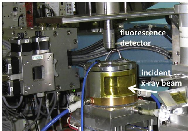
**Fig. 3.** Cylindrical sample cell with Kapton windows used in the experiment. The incident X-ray beam enters from the right, as shown by the arrow. During the experiment the fluorescence detector is lowered close to the liquid surface.
