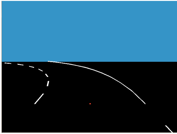
(a) In the sensor layout depicted by Fig 3, a vision-based approach is used to detect the lane markings. The input data can be grabbed directly from the 3D simulation environment.
