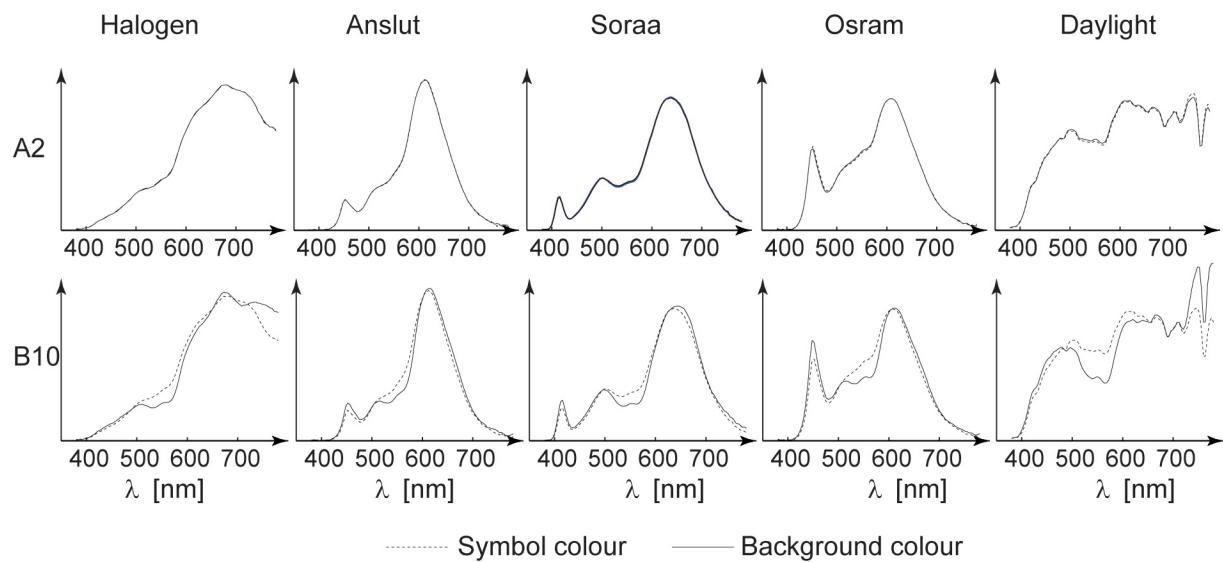
**Figure 4 – SPDs of the reflected light from symbols A2 and B10 and their backgrounds, under different illumination.**
