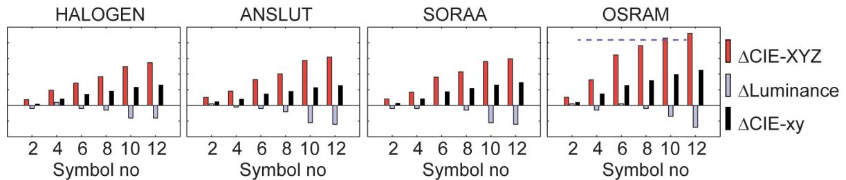
**Figure 6 – Histogram of measured colour difference at row B. The dotted line indicates the identification threshold. Symbol 10 was possible to identify for all observers with normal colour vision, in Osram illumination.**
