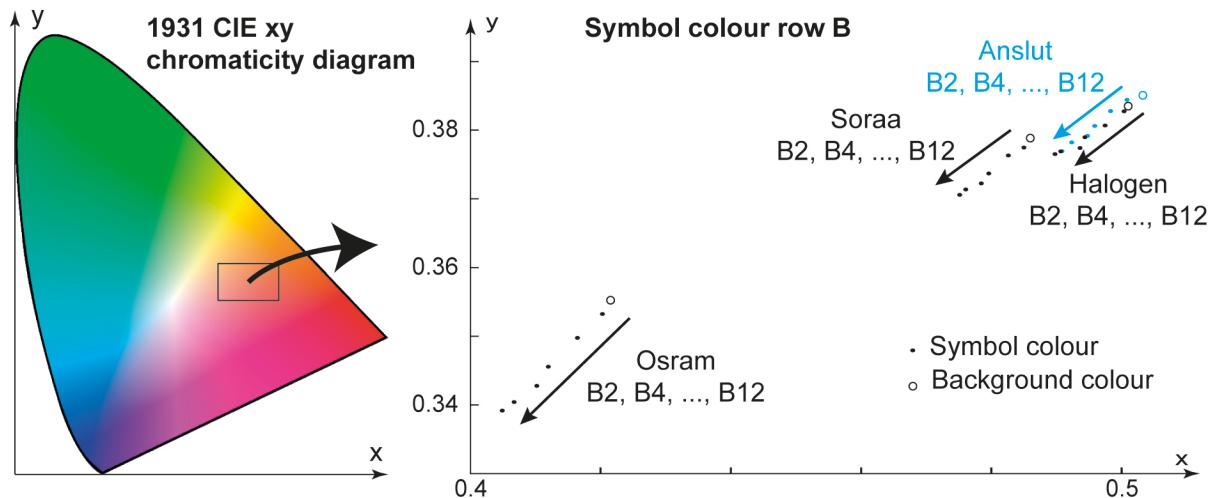
**Figure 5 – CIE-xy chromaticity coordinates for symbols B2, B4, B6, B8, B10, B12 and background colour under illumination by four light sources.**
