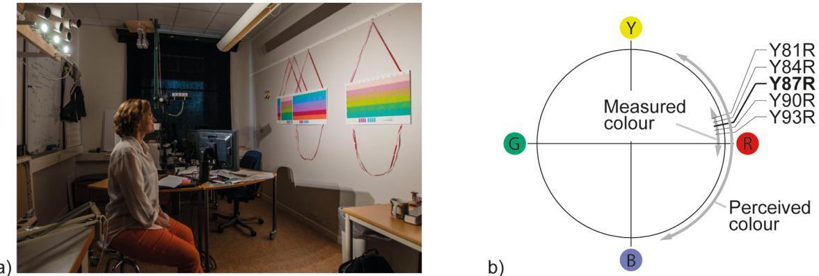
**Figure 1 – a)** View inside the test room. **b)** NCS Colour Circle with the first five hue values for row B marked in the colour contrast chart. The difference between measured and perceived colour is also illustrated.
