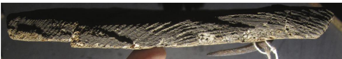
Fig. 10. Cleaved board from the Hammarö Church. The Hammarö church trefoil board SHM 23700:6. Note the almost horizontal growth rings, which strongly indicate that four boards were produced from one timber. Photo Karl-Magnus Melin.
