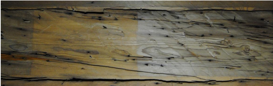
Fig. 9. Roof board from the Tångeråsa church. The board has very warped fibres. It was necessary to use a controlled cleaving technique to succeed with a tree like this. This type of material was tested, with good results, in the practical experiments. Photo Christina Persson.
