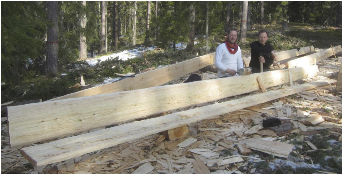
Fig 23. Boards resulting from a successful cleaving. Note that all of the boards are of the same length in all photos. Photo Mattias Hallgren.
