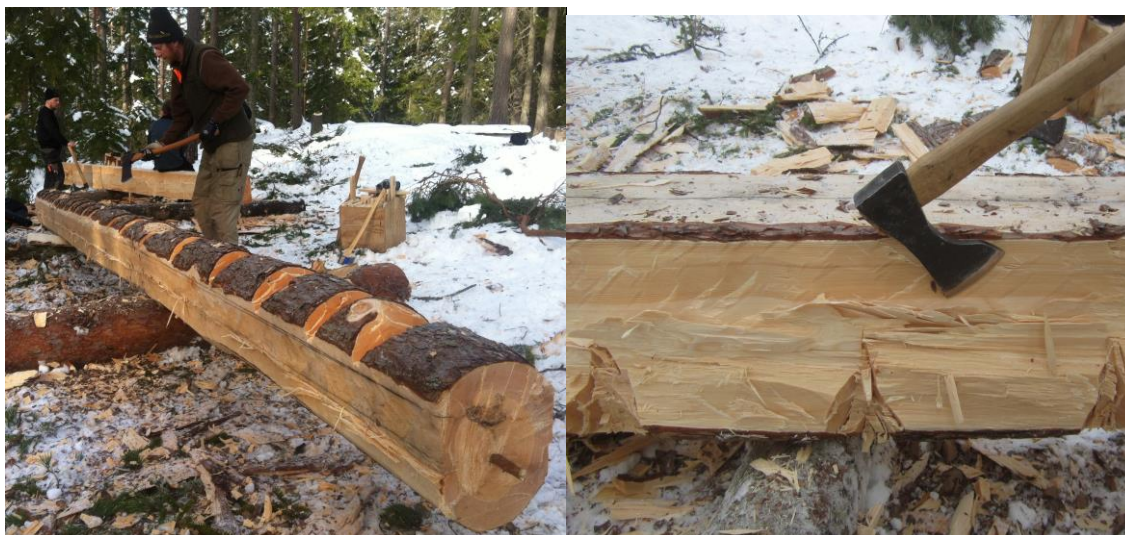
Figs. 15–16. Boxing the log. To box the logs, first the corners were marked with soot lines and then the log was turned and scores were made about one to two feet apart, almost touching the soot lines. Then the log was turned back and the segments were cut and cracked away ( klamphugg ). Photos Ola Hugosson and Karl-Magnus Melin.
