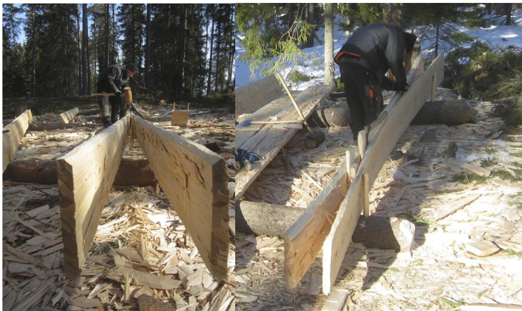
Fig. 19–20. Grooving. The cleaving technique was improved by making a v-shaped groove. Remains of the groove can be seen in the picture. The grooving was only done on the second (tangential) cleaving in order to minimise the risk of cracking the thin boards produced. In the picture on the left, the cleaving is made from one end to the other. The one on the right shows the cleaving made from both ends simultaneously. In the experiments made in 2014 and 2015 we have rationalized the grooving procedure away since we on these later occasions did not cleave frozen wood. Photos Karl-Magnus Melin.
