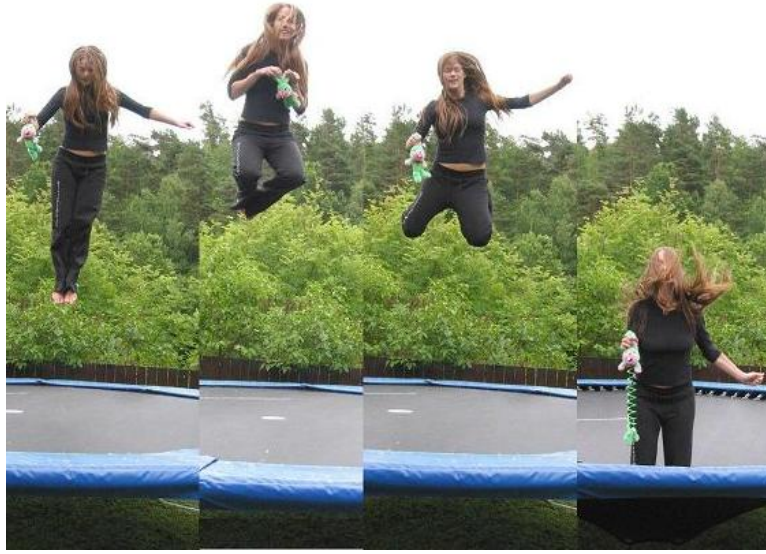
Figure 1. A spiral toy used as accelerometer during a trampoline jump. Note how the spiral in the toy is contracted while the jumper is in the air, and expanded at the bottom of the jump. Also note how far down the trampoline is displaced in the last photo.
