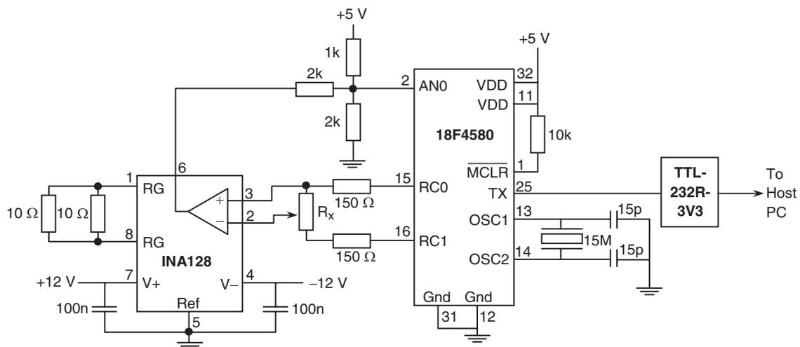
FIG. 8. The digital milli-ohmmeter hardware.
