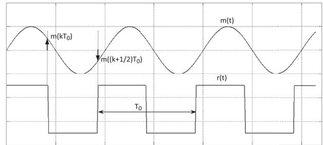
FIG. 3. Firmware PSD: Take samples separated by  $0.5T_0$  and subtract pair-wise.<sup>15</sup>
