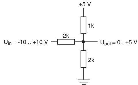
FIG. 6. Bipolar-to-unipolar converter.<sup>21</sup>
