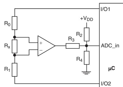
FIG. 4. Digital lock-in amplifier for sub-milliohm measurements.
