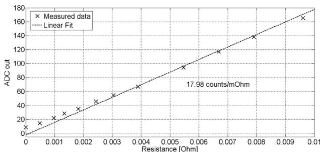
FIG. 10. The detector is less sensitive at the low end.
