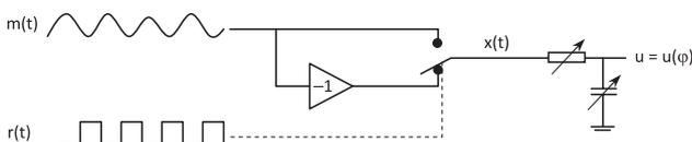
FIG. 2. Phase sensitive detector.
