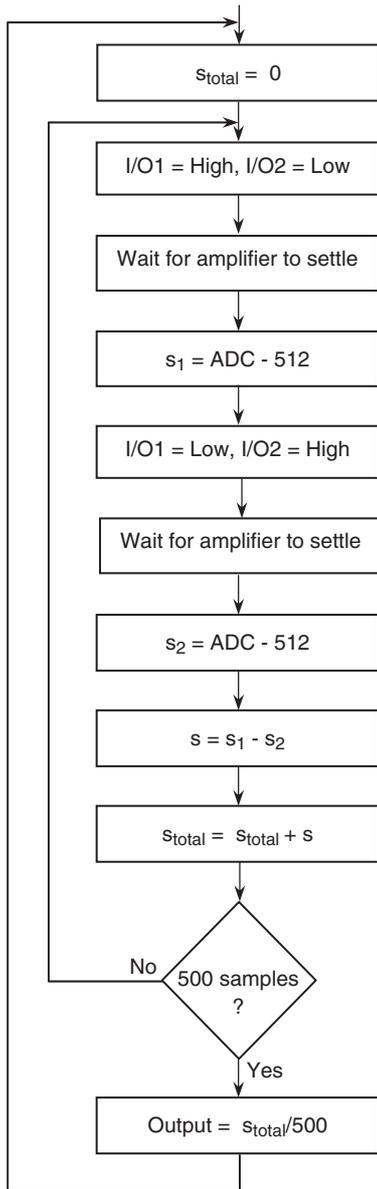
FIG. 5. Digital lock-in amplifier: Firmware flowchart.
