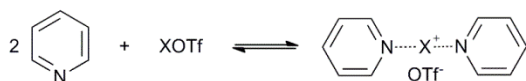
Scheme 1. Hypothetical reaction for estimation of the stability of complexes 1-3 . The predicted energies (DFT) are shown in Table 2.
