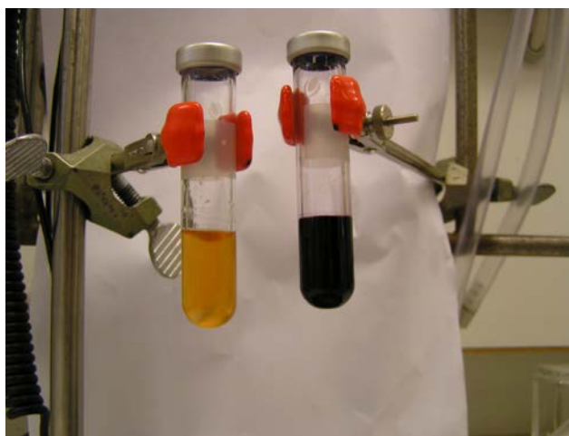
Figure S1. Microwave vials charged with the catalytic system: (a) Pd(OAc) 2 (5 mol%), P( t Bu) 3 (8 mol%) and NaO t Bu (140 mol%) in α,α,α-trifluorotoluene (yellow solution on the left), and (b) Pd(OAc) 2 (5 mol%), P( t Bu) 3 (8 mol%) and sodium 2,4,6-tri- tert -butylphenolate (140 mol%) in α,α,α-trifluorotoluene (deep purple solution on the right).
